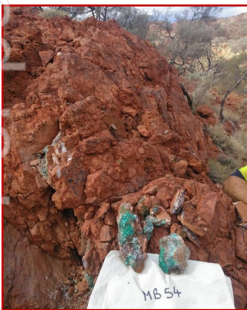
Photo 1. Rock chip sample MB54; 15.2% Cu & 0.16 g/t Au
