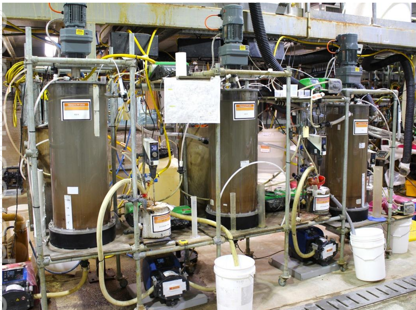
Figure 2: Counter Current Decantation (CCD) Wash circuit
