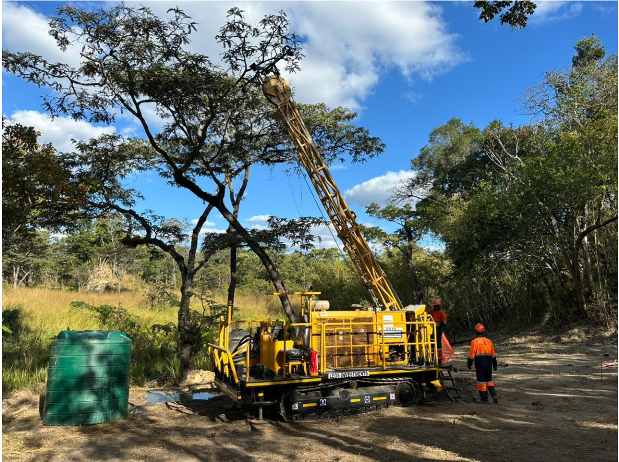
Figure 2. Diamond drilling being completed for the Kabikupa deposit at Mumbeshi Copper Project
