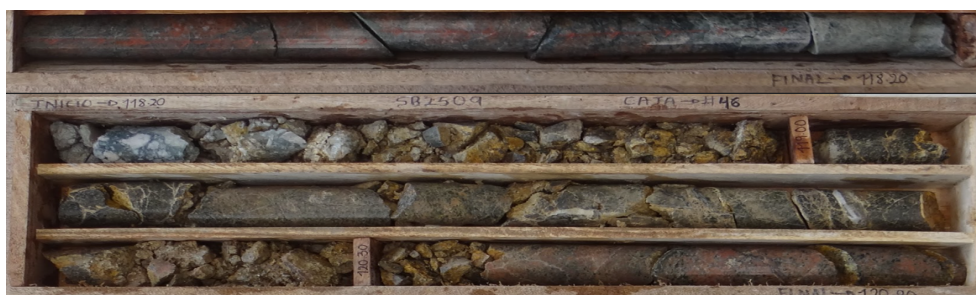
Photo 3. Drill Hole SB-25-09, Mariana Vein #1 intersection from 118.2 to 118.6m. The vein is faulted, broken, weathered and oxidized due to proximity to surface. Sample DH020062.
