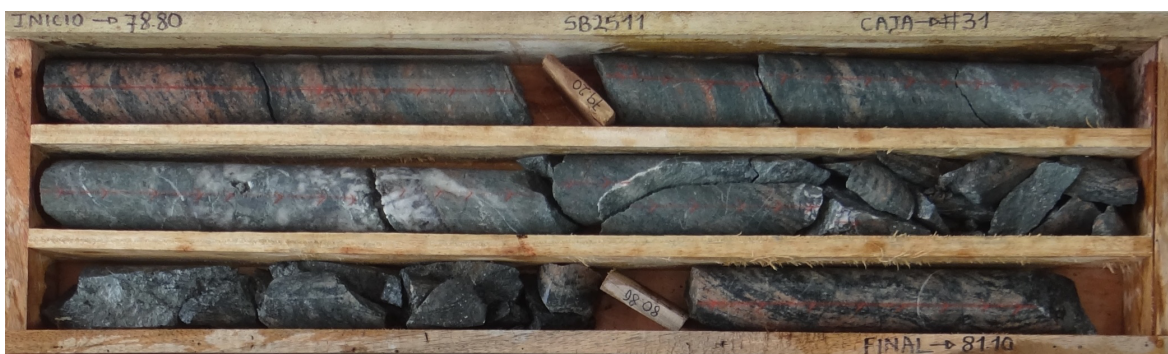
Photo 5. Drill Hole SB-25-11, Vein #1 intersect from 79.65 to 80m ( 18.9 g/t Au and 22.5 g/t Ag, Sample DH020057) comprised of Stages 1 and 2 quartz with up to 15% Pyrite, 5% Arsenopyrite, 5% Sphalerite and 2% Galena) with pervasive sericite/chlorite haloes in both hanging wall and footwall, this last including Stage 2 quartz veinlets.
