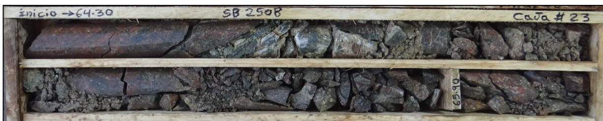
Photo 2. Drill Hole SB-25-08, where a fault zone is affecting the target Mariana vein (middle of upper row), still preserving quartz vein fragments. Sample DH020093 from 65.05 to 65.9m)
