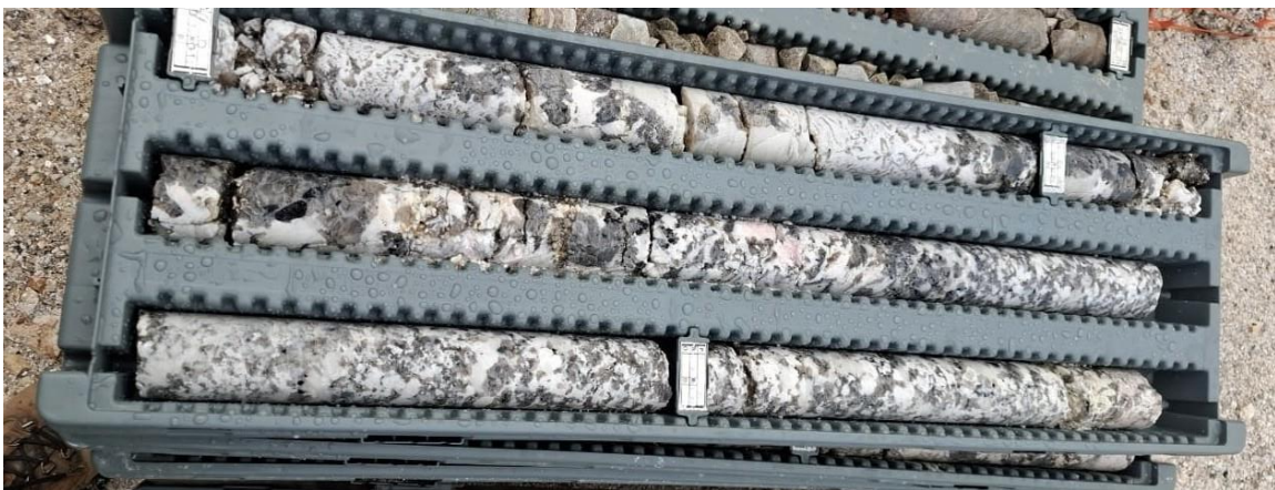
Figure 7: Drill core from hole PMB25-04, showing a pegmatite section from 3.3 to 6.2 metres downhole.
