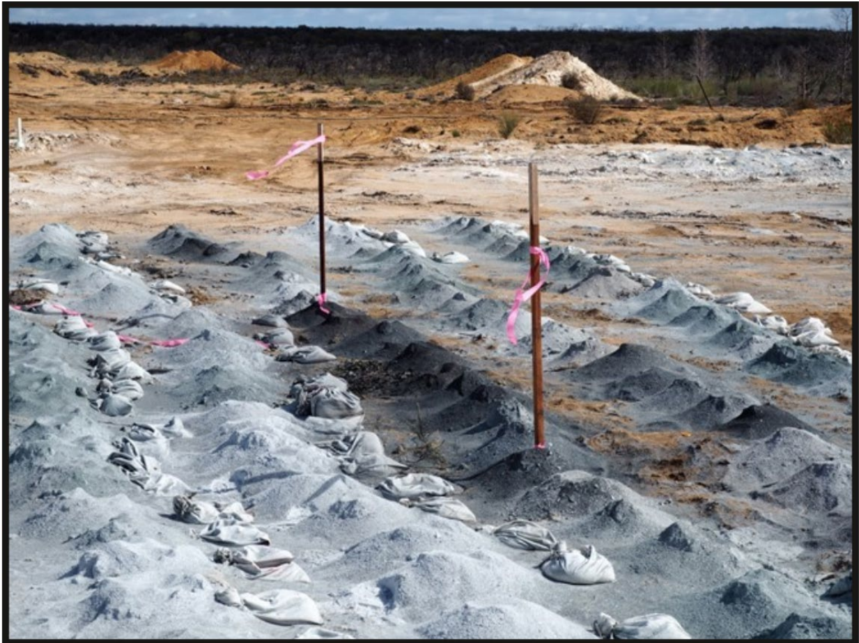
Figure 12 - NRRC0124 R/C Drill piles, black material represents massive sulphide intersections (128-138m marked by wooden pegs).
