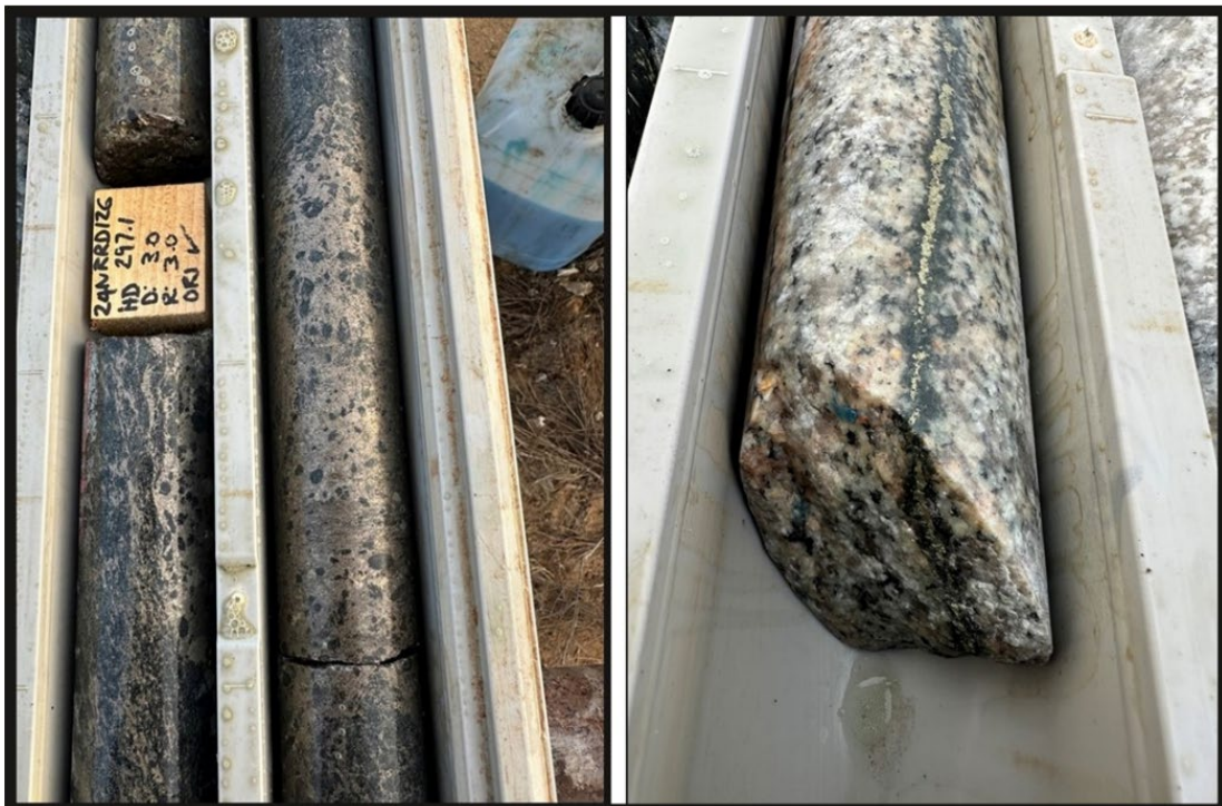
Figure 13 - Massive (left) and veined (right) sulphide mineralisation within hole NRDD0126 contained within interval 295.1 -300.3m (5.2m).
