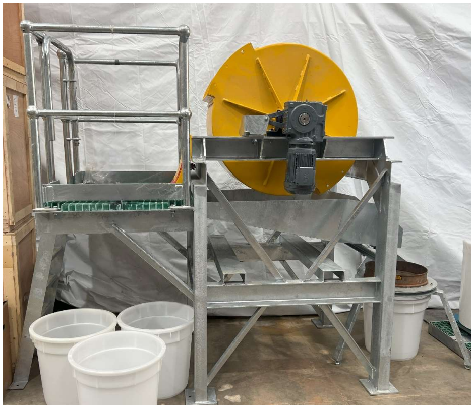
Figure 1 – Pilot Plant Scrubber
