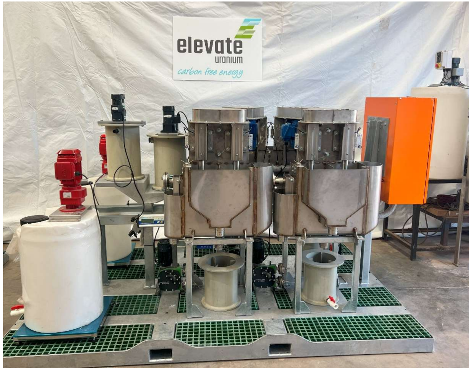
Figure 2 – Pilot Plant Calcite Removal
