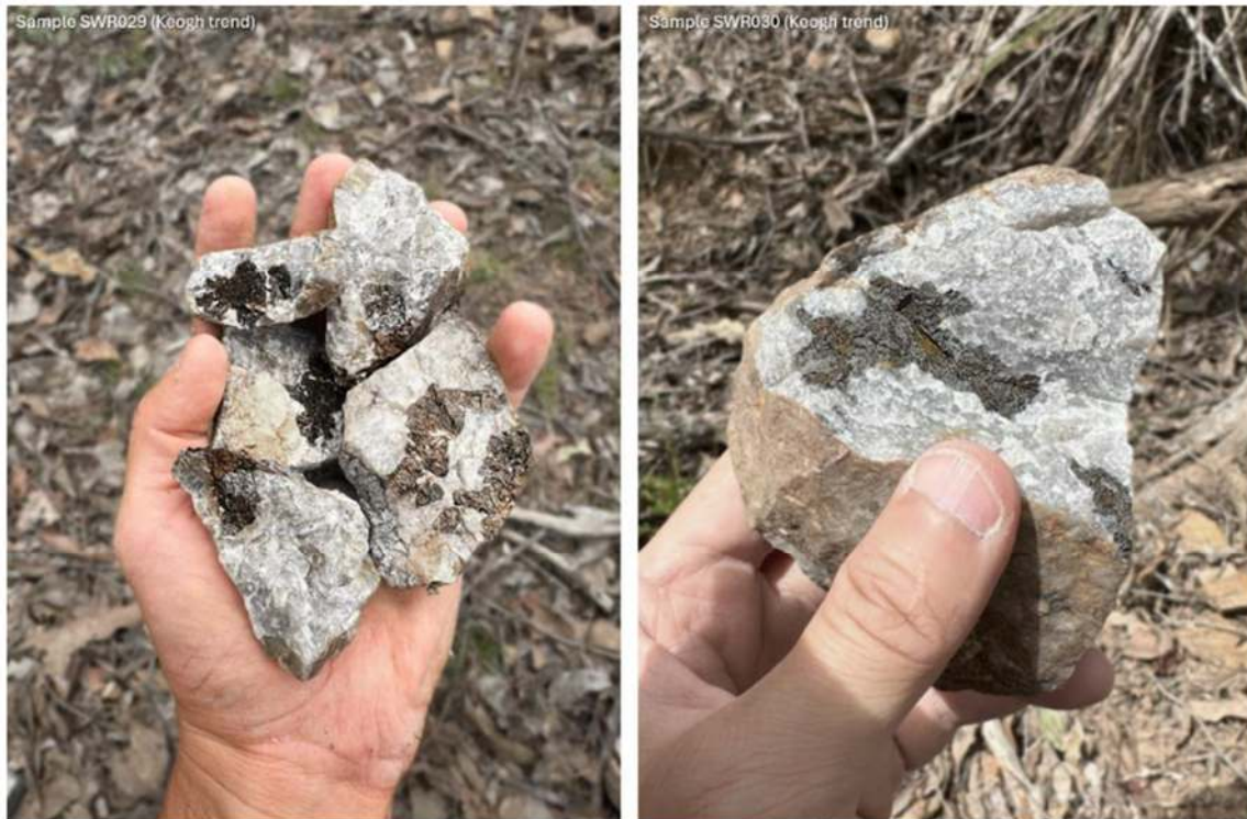
Figure 15 - Care cassiterite (tin-oxide) dark mineral crystals and aggregates, from the Sweetwater area: L) Sample SWR029 (16.70% SnO 2 ) and R) Sample SWR030 (8.65% SnO 2 )
