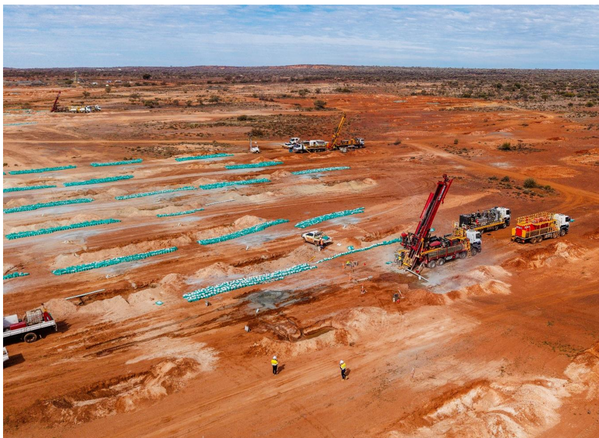
Figure 1 - Three Rigs undertaking Infill Drilling at Mt Ida (view to south)
