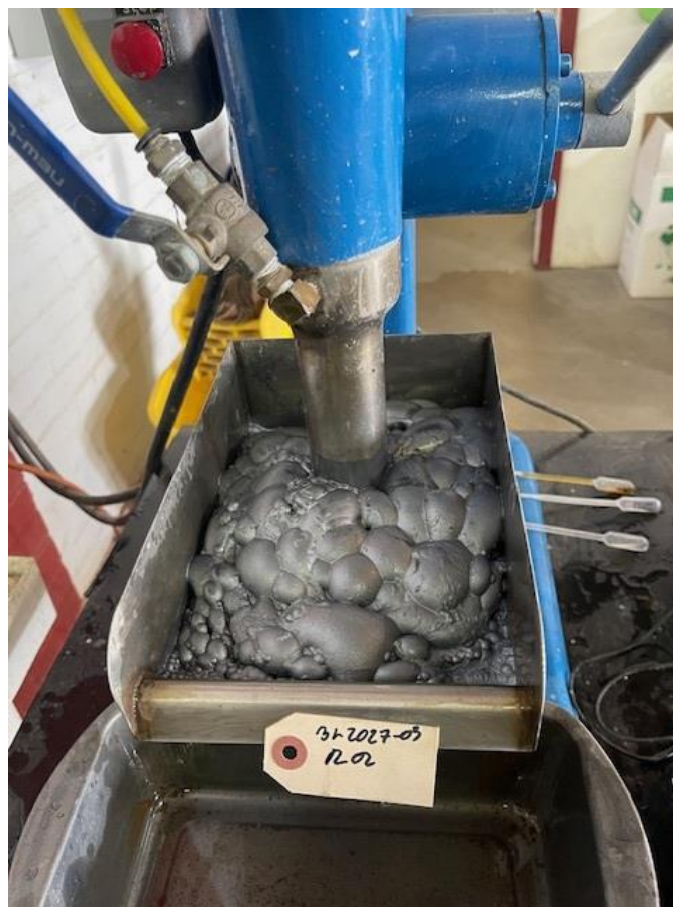
Figure 2; Photo of flotation testwork underway on test R02. Note grey colour of the bubbles is due to stibnite.
