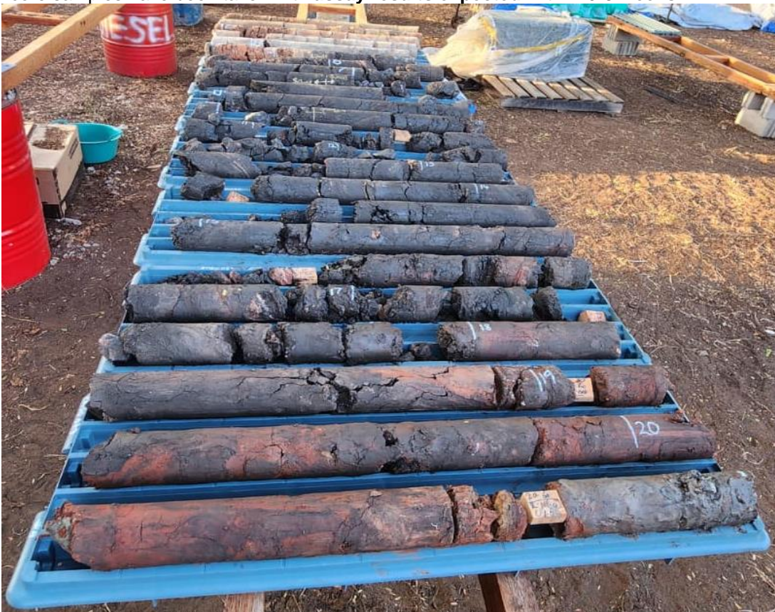
Figure 1: Secondary manganese in core from EMDD033, looking from the bottom of the hole. For visual estimates and visual estimates disclaimer please refer to table 1.
