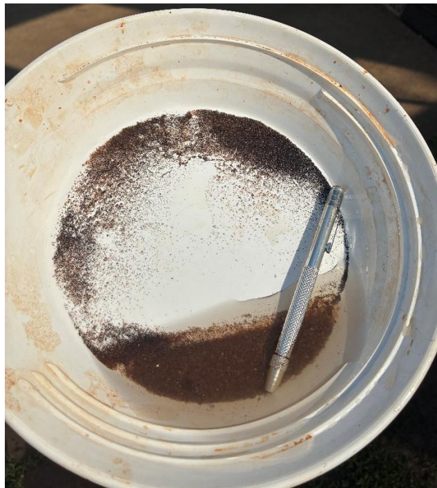
Figure 2. Rutile in a panned alluvial sand concentrate from soil sample SS118 at Mkanda Rutile Project. The soil sample was taken from surface and panned to a concentrate for mineral identification. Estimated in-situ rutile grade range within the sample of 0.75% - 1.5%. See cautionary statement under Figure 2.
