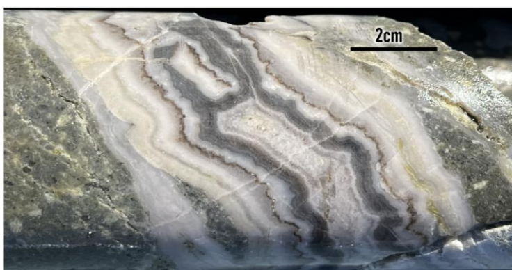
Figure 6: Colloform (A) – crustiform (B) quartz-adularia vein with black silica banding in interval from A Vein in 25FCDD002.
