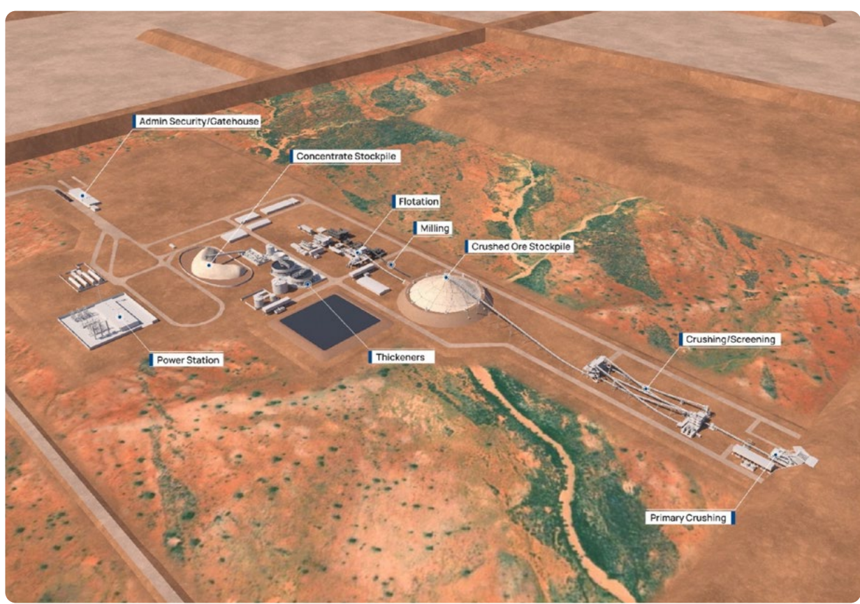
Figure 4: Process plant layout for the Tabba Tabba Project.
