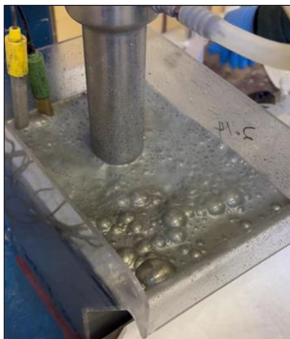
Figure 10: Flotation tests producing rougher concentrate
