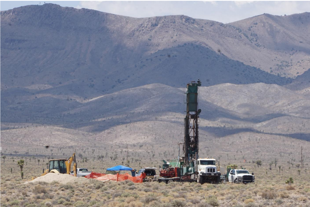
TRUCK MOUNTED RC DRILL RIG ON SITE DURING ALKALI FLATS PHASE 2 PROGRAM
