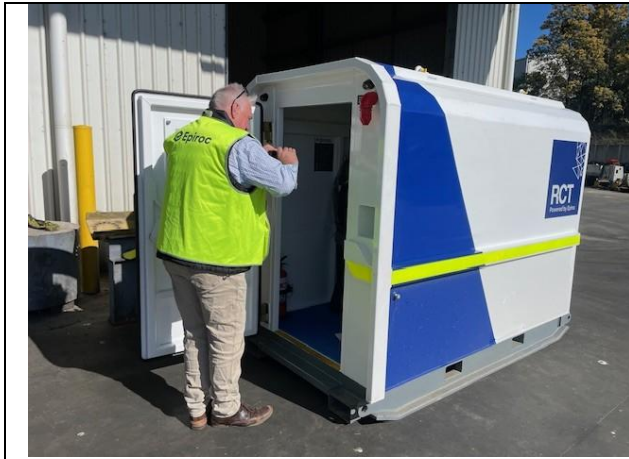
Figure 7 – Remote control chamber
