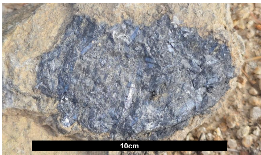
Figure 2: A rock sample collected from a historical mine located at the Antimony Ridge Target. Refer to Appendix B for sample locations. The photo shows a single rock specimen comprising the grey-silver coloured metallic mineral stibnite. Stibnite is an antimony sulphide ore mineral, containing 71.7% mol weight antimony. The stibnite in this rock specimen is massive, containing between 75% and 90% stibnite. Coarse to very fine stibnite crystals are visible which form an interwoven mass. Visual estimates also potentially provide no information regarding impurities or deleterious physical properties relevant to valuations. Samples similar to this photographed rock specimen have now been assayed. As reported in this announcement the results are as follows: 730253: 49.8% Sb and 1,420 g/t Ag and 3.12 g/t Au. PLEASE REFER TO THE FOLLOWING SECTION FOR STIBNITE V'S SB %'s.
