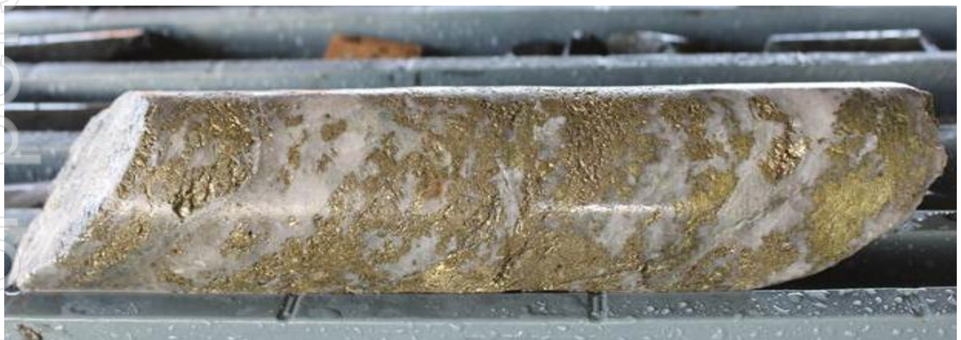
Figure 3 - The main quartz-carbonate-pyrite-chalcopyrite vein with strong sericite-chlorite selvages of the Displaced Lode mineralisation in DTDD056 (143.5 – 143.9m).
