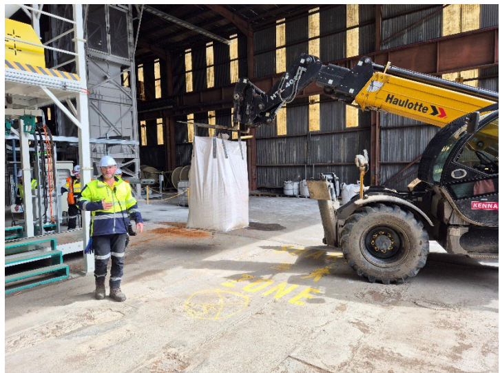
Loading of MgO into 1t bags (left) and relocating bags to storage area (right)
