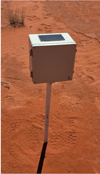
Figure 2 (left): An IVY hydrogen sensor deployed on site 4.
