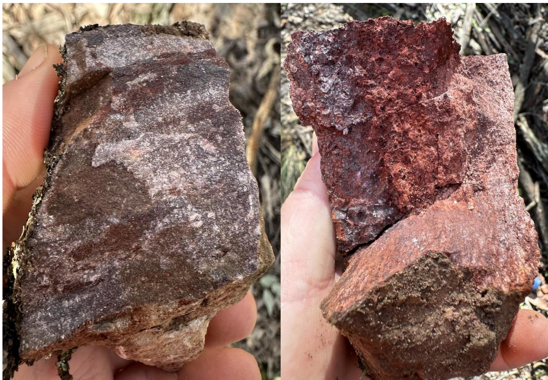
Figure 20 – Silver mineralisation within ferruginous barite outcrop yielding 117 g/t Ag, & 0.26% Ba from sample 3001009
