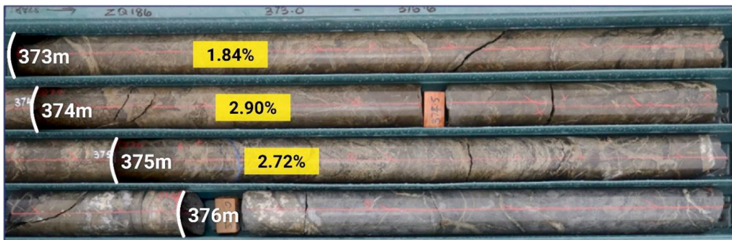
Figure 8: Drill core from ZQ186, 373-376m down hole showing high-grade interval from 374 to 376m averaging 2.81% Sn
