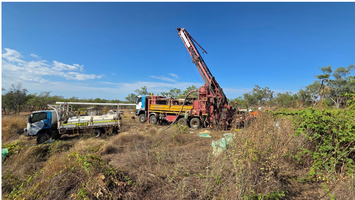
Figure 2: RC drilling underway at Electric Light
