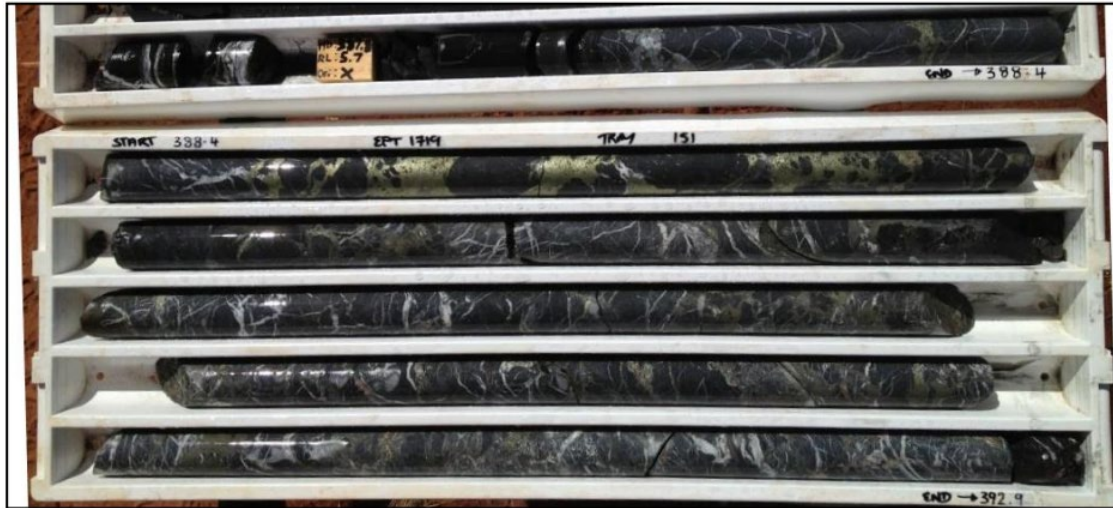
Photo 1: EPT1719 - ~387.6m to 392.9m (5.3m @ 2.5% Cu) – Veined and brecciated carbonate with local massive copper sulphide breccia cement 3
