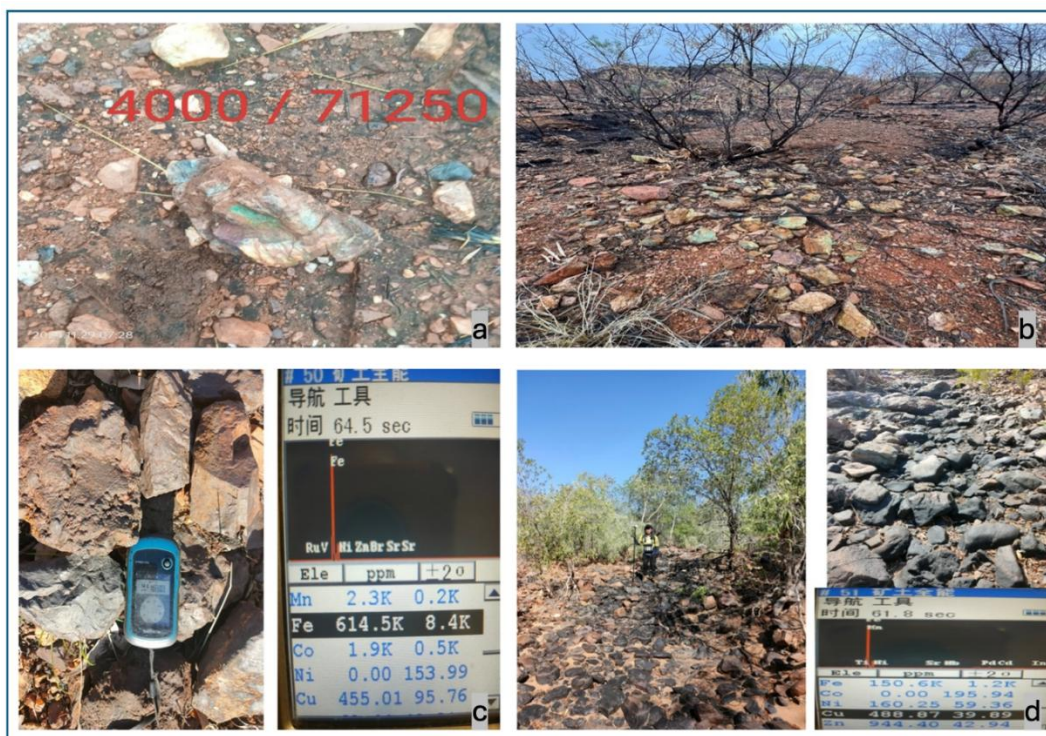
Figure 4: Photos illustrating high grade oxidized copper ore, mainly malachite (a, b), magnetite quartzite (c) and meta-mafic unit). Note that P-XRF analyses reading are indicative only for guiding further test work.
