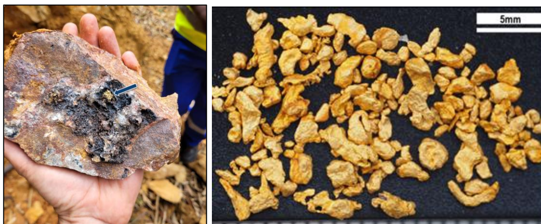
Figure 2: In situ gold in veining at A1 drill pad (LHS) and artisanal gold grains from Binda artisanal working (RHS).
