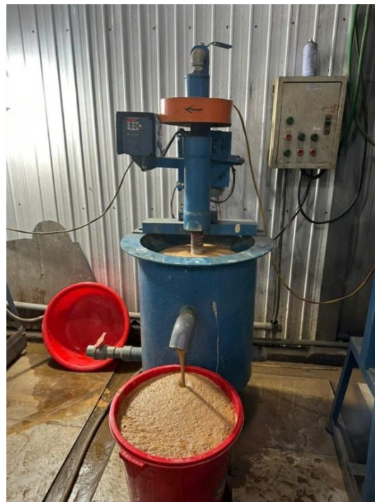
Image 1 - Flotation cell used for the treatment of the bulk sample
