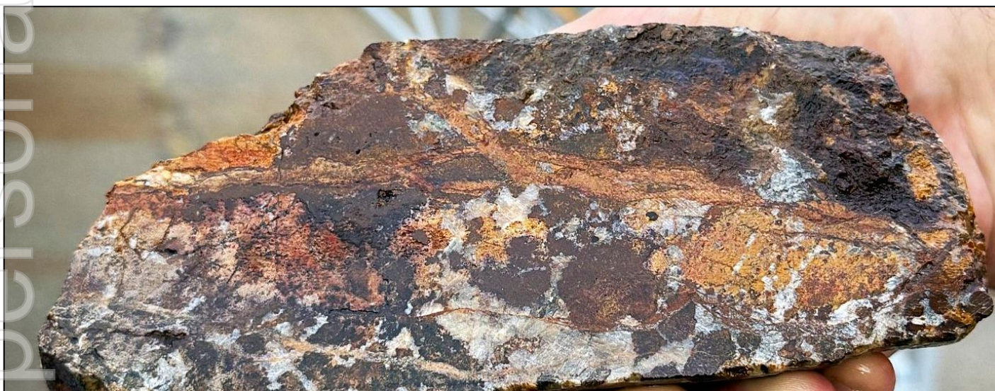
Figure 6. Core photograph from 229.5m to 231.7m in ZRSD25195 showing pyrite, sphalerite and chalcopyrite – 10.1g/t Au and 0.2% Zn.
