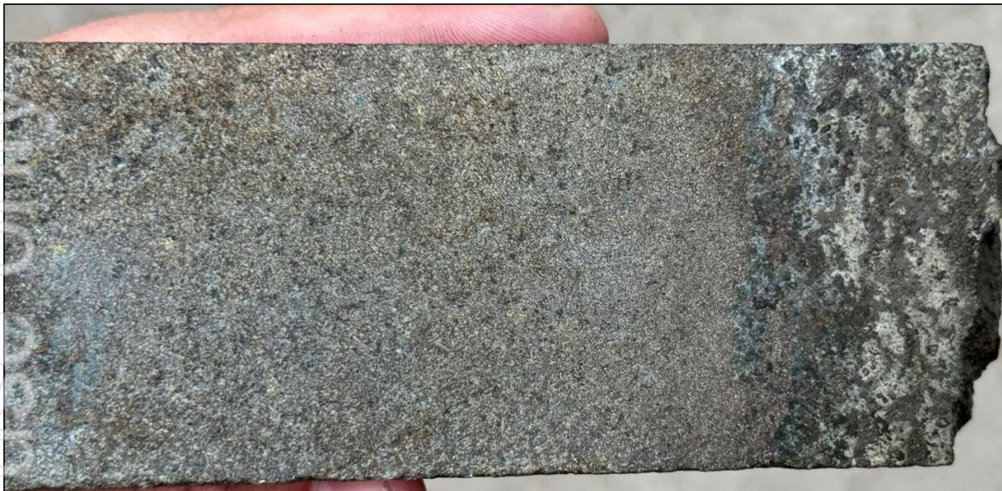
Figure 5. Core photograph from 485.0m to 487.0m in ZRSD25193 showing strong pyrrhotite alteration – 5.5g/t Au.
