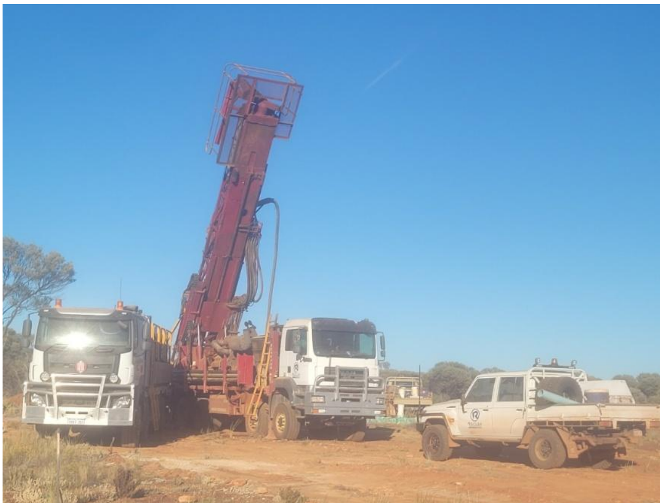
Figure 1: RC Drilling Rig onsite Mulgabbie North Cross Fault
