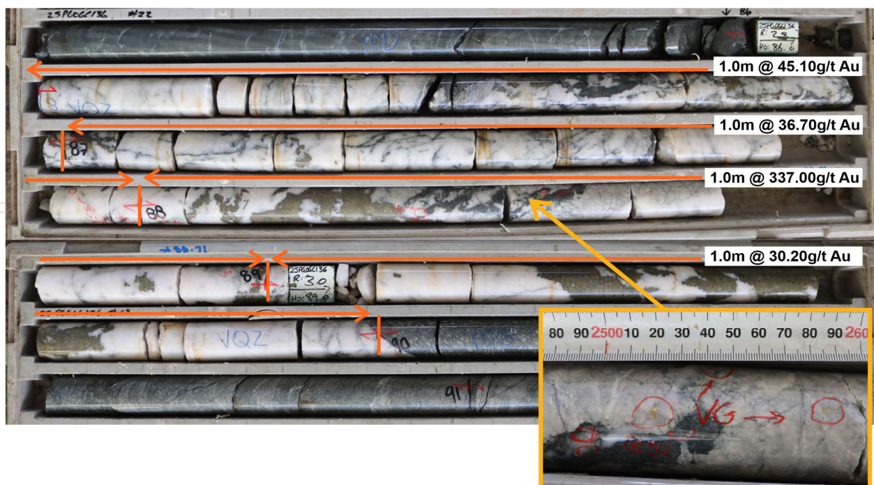
Figure 1: Core Photo of 25PGOGC25136 showing the 5m @ 90.55g/t Au interval with the sub-sample intervals indicated.
