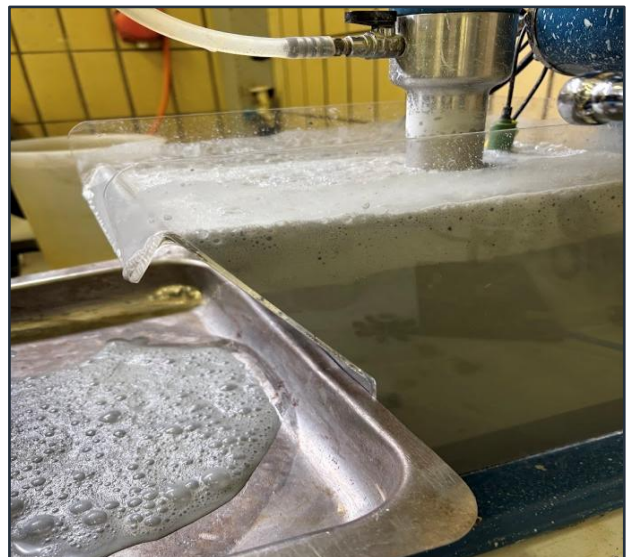
Figure 5: Rougher flotation (medium- and slow-floating PGM fraction)
