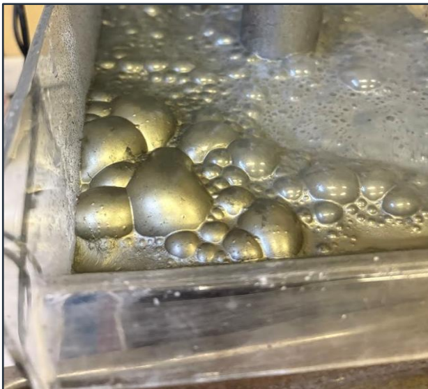
Figure 4: Flash flotation (fast-floating PGM fraction)
