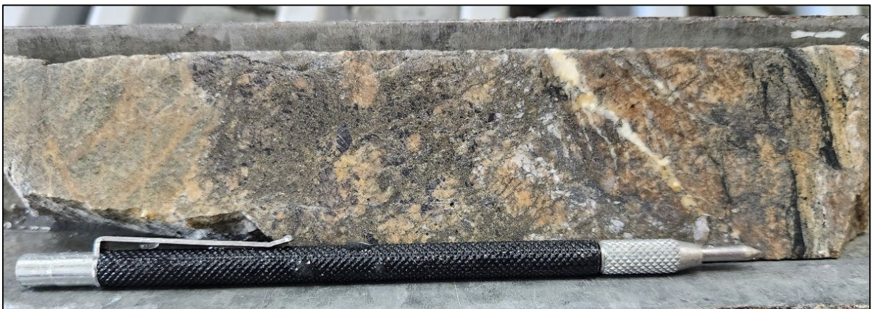
Figure 2 – Mineralised carbonate-pyrite-arsenopyrite-cobaltite-scheelite vein (2019FTD007E, 129.8m) (Interval 129.5-130.0m Assay: 0.5m @ 6.64g/t Au, 0.38% Co, 1.02% WO 3 , 0.11% Cu ).
