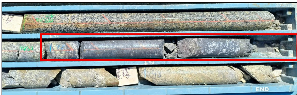
Figure 1 - High-grade stibnite from Drill Hole CBADD001 showing massive sulphide, highlighted in Red, from 42m downhole. Estimation* of sulphide content is approximately 70% Stibnite, with assays expected to be returned in Early November.
