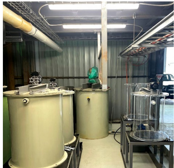
Figure 3 - Demonstration Plant – Iron oxidation and precipitation circuit (left) and installation of iron polishing and MHP precipitation circuits (right).
