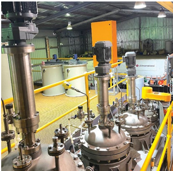
Figure 3 - Demonstration Plant – Iron oxidation and precipitation circuit (left) and installation of iron polishing and MHP precipitation circuits (right).
