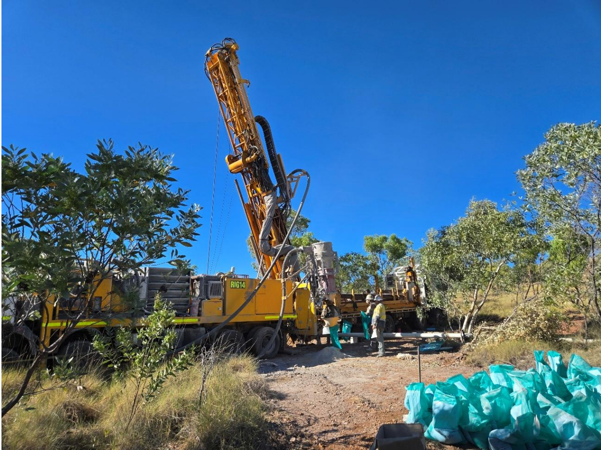
Figure 3: Aruma’s RC drilling at the Piper Prospect, Fiery Creek project
