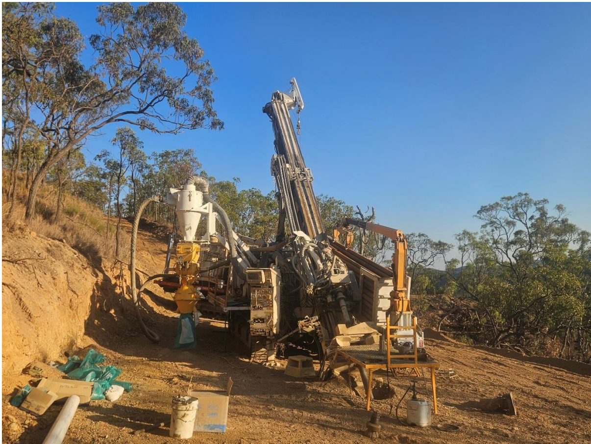
Figure 1 RC rig drilling first shallow VTEM Target hole (ORR 128)
