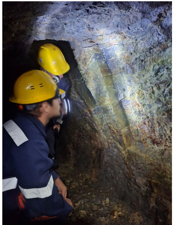
Photograph 1 and 2: (Left) Exposed antimony rich vein within adit 80 were 2014 channel sample #2010_V-6_A80_2014 which returned 22.6% Sb and 3.23g/t Au from the 70cm channel. (Right) Krakatoa geological team inspecting the adit and channel sample cuts.
