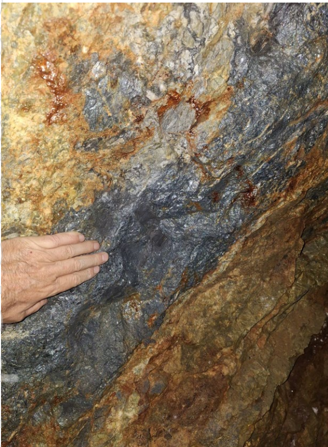
Photograph 1 and 2: (Left) Exposed antimony rich vein within adit 80 were 2014 channel sample #2010_V-6_A80_2014 which returned 22.6% Sb and 3.23g/t Au from the 70cm channel. (Right) Krakatoa geological team inspecting the adit and channel sample cuts.
