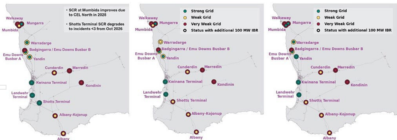
Figure 2: 2025 ESOO: System strength outcomes – Oct 2024 (left), Oct 2027 (middle) and Oct 2031 (right) 6
