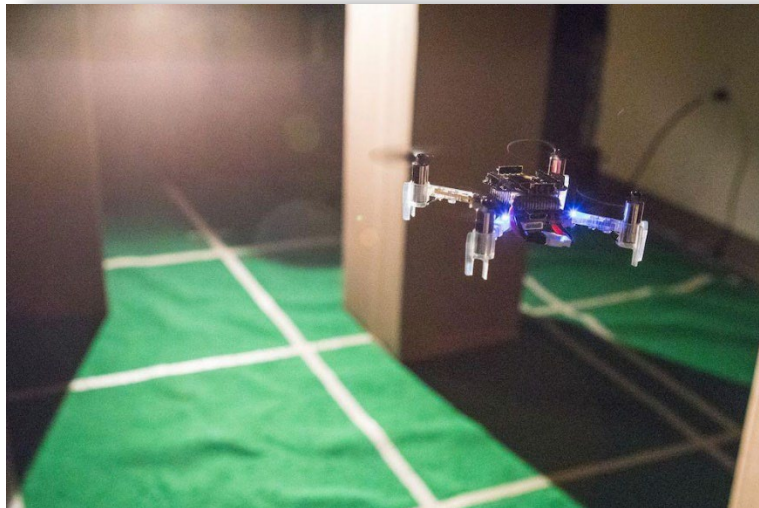
Figure 1: Image of the Crazyflie 2.1+ drone, a versatile open-source flying development platform that weighs 29g to be used in the upcoming live drone testing.
