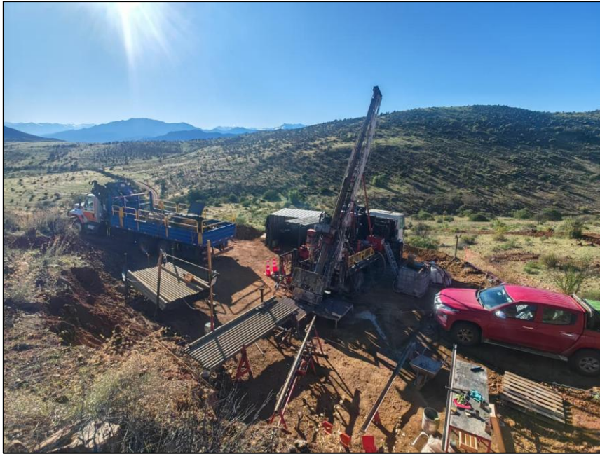
Figure 6: Drill rig drilling maiden diamond hole CMQD001 at El Quillay West.
