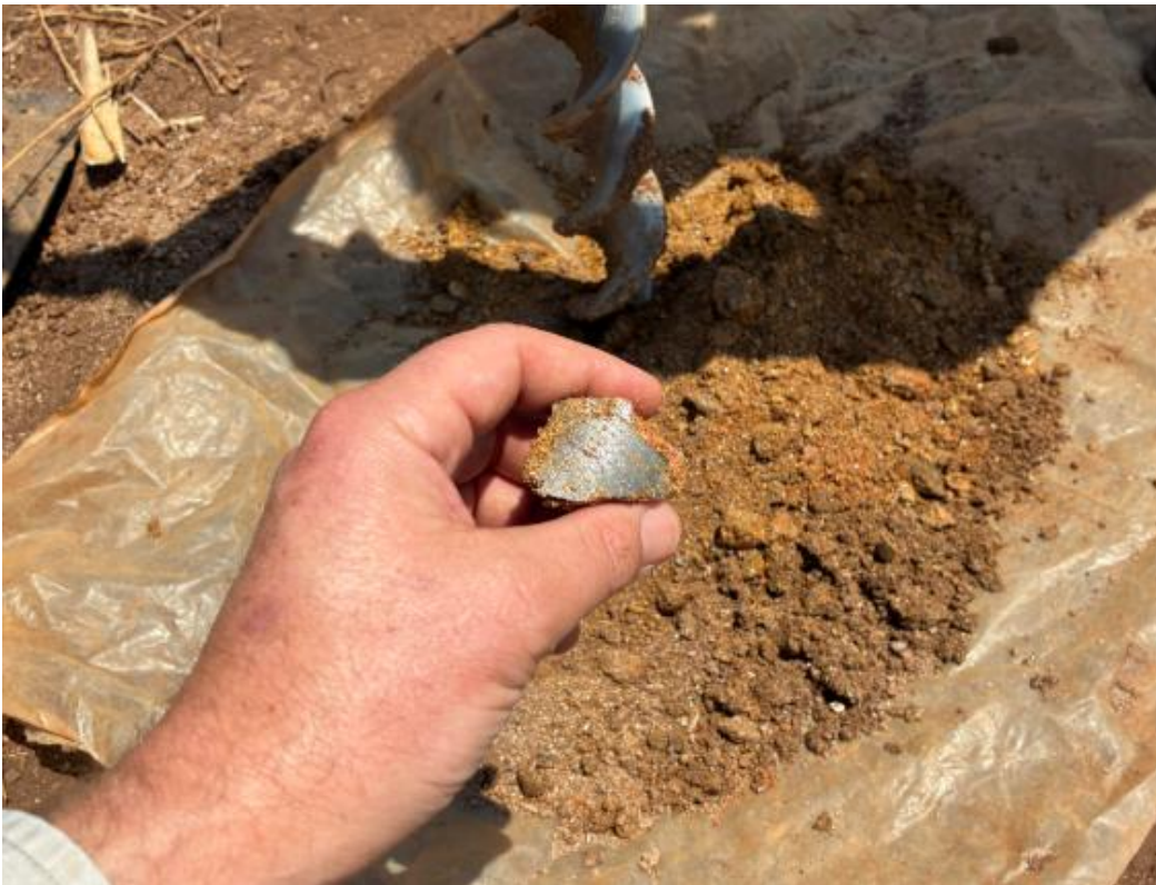
Figure 3. Graphite mineralisation observed in Fortuna's first drill-hole MHA0001 in soft friable saprolite. Refer to Appendix 1 for further information.
