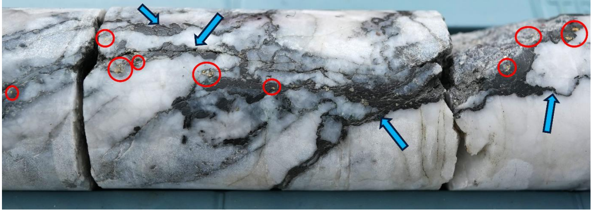
Figure 7 BMDD001W6 showing visible gold (red circles) and stylolites (blue arrows) in the NQ core (47.6mm diameter) from 832.7 to 832.9m
