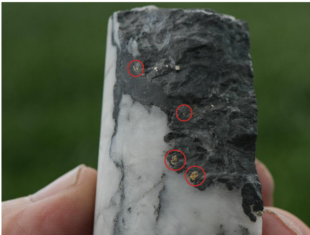
Figure 10 Visible gold in NQ core (47.6mm diameter) in BMDD001W6 at 832.9m
