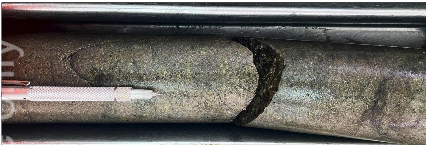
Figure 6. Core photograph from sample interval 195.3 to 196.0m in ZRSD25214, showing massive chalcopyrite and pyrrhotite mineralisation – 3.9g/t Au and 5.6% Cu.
