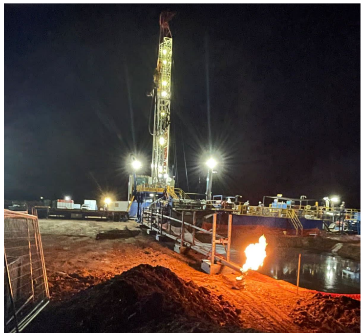
Figure 1: Controlled flare of circulating gas from Diona-1 well
