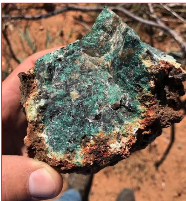
Figure 2: Quartz-chalcocite filled vugs in Cromwell A shear zone with malachite rosettes ( \pm 5-12\% visual est.) intergrown with chalcocite ( \pm 2-4\% visual est.) [assay not yet received]
