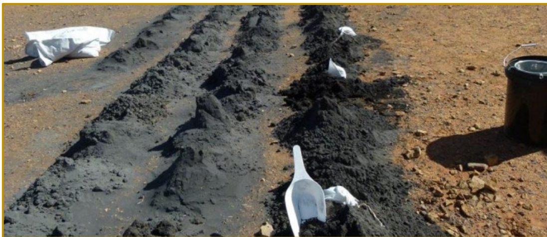
Figure 2. Sample spoils of black shale from previous RC drilling at the Byro Critical Minerals project
