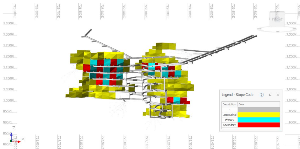
Figure 8 Sulphur Springs's stope mining methods
