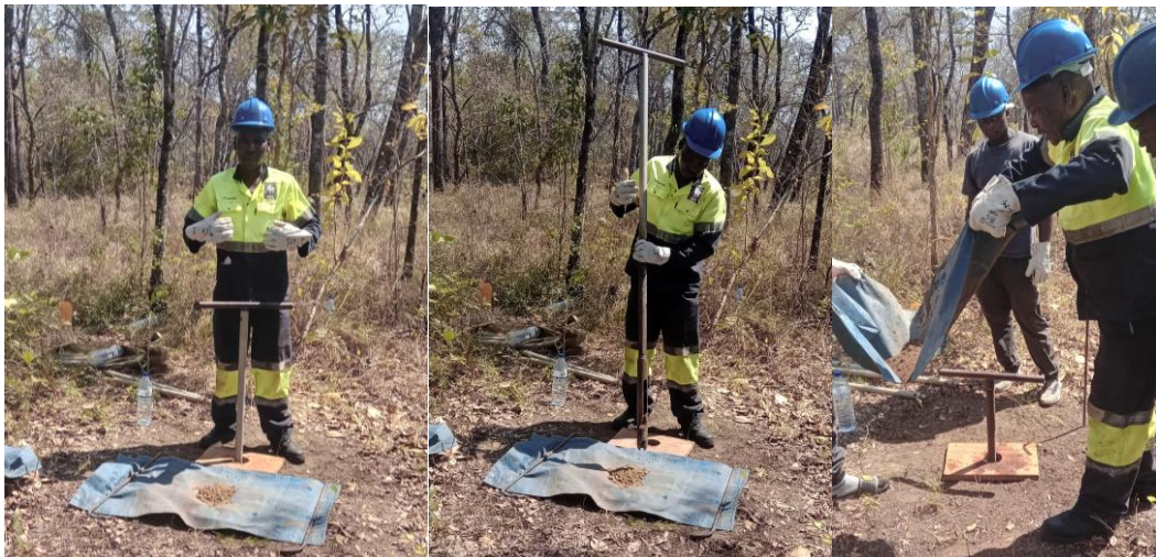
Figure One: Field technicians conducting hand auger drilling at the Adriano rare earth licence in Mozambique. The team is testing for potential alluvial rare earth element (REE) deposits in proximity to previously identified high-grade stream sediment anomalies.
