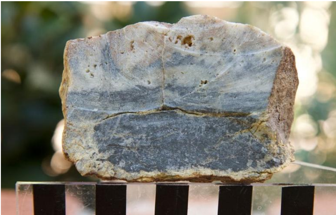
Figure 4: Photograph of rock sample TJ25ROC2 showing the banded Quartz-Stibnite vein (sample is ~7cm across)
